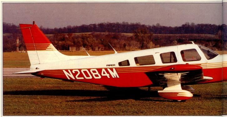
Piper also made the Six a retractable in 1976, calling it the Lance. Two years later, the Lance would sport a T-tail—which contributed to comparatively lackluster runway performance—and plummeting sales numbers.
